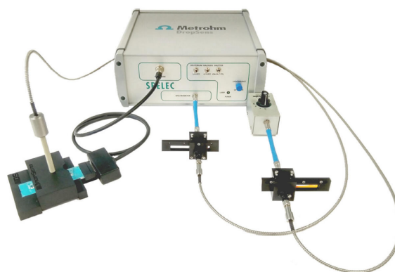
Figure 1. Fluorescence spectroelectrochemistry setup used for the study of Alamar Blue.
