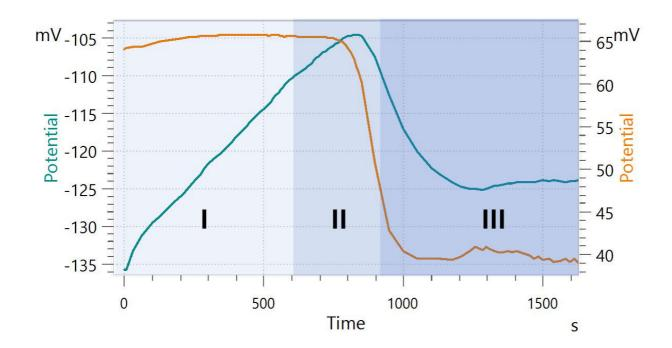
**Figure 2.** Example curve for calcium carbonate formation. In green is the potential of the free calcium ions measured with the combined Ca ion-selective electrode, and in orange, the potential measured with the Optrode. The experiment was carried out at pH 11. The colored phases describe the prenucleation phase (I), nucleation (II), and particle growth (III).
