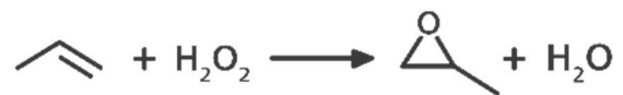
Reaction 1. Overall reaction for the epoxidation of propylene with hydrogen peroxide (HP-PO).
