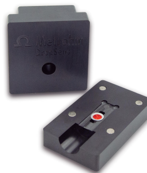
Figure 1. Raman spectroelectrochemical cell.
