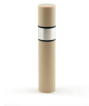
Figure 1. Rotating cylinder electrode showing the metallic insert, the Viton O-rings (black) and the PEEK holder.
