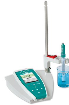
Figure 1. 913 pH Meter equipped with a pH electrode. Example setup for the determination of the pHe value.
