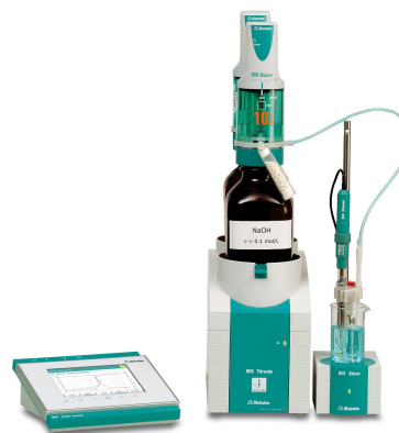
Figure 1. 905 Titrando equipped with a Solvotrode easyClean for the analysis the epoxide equivalents controlled by a 900 Touch Control.
