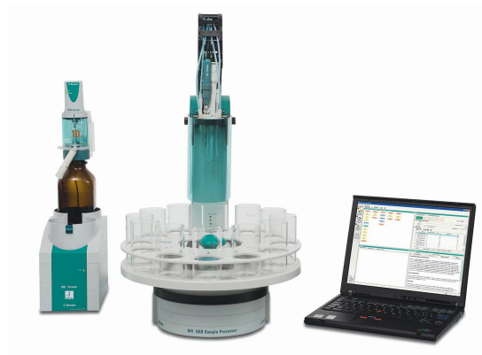
Figure 1. 814 Sample Processor and 905 Titrand equipped with an iAg-Titrode with \text{Ag}_2\text{S} coating controlled by tiamo software.
