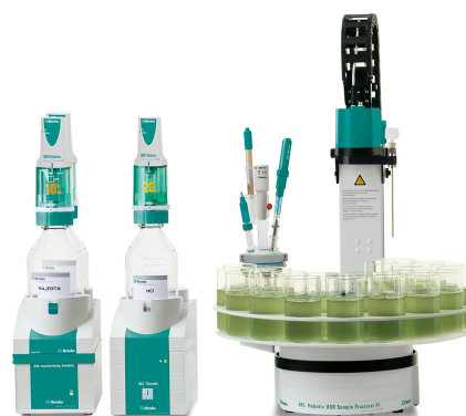
Figure 1. Example system: 815 Robotic USB Sample Processor XL with an external titration vessel, 905 Titrande and 856 Conductivity Module equipped with iAquatrode plus, iAg-Titrode, and 5-ring conductivity measuring cell for the analysis of tap water.
