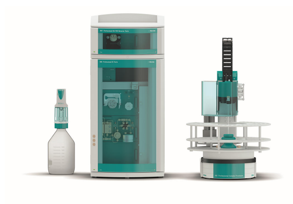
Figure 1. Instrumental setup including a 940 Professional IC Vario (center), 947 Professional UV/VIS Detector Vario SW (top center), 858 Professional Sample Processor (right), and MiPCT-ME, performed with the Metrosep A PCC 2 HC/4.0 and Dosino (left).
