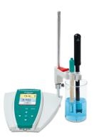
**Figure 1.** 914 pH/DO/Conductometer equipped with an O2-Lumitrode, conductivity measuring cell, and iUnitrode (missing in the picture) for the determination of DO, K (conductivity), and pH in liquid dairy products.
