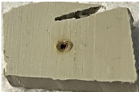
Figure 5. Example of sample burning with a 1064 nm system. This material was identified as polyphenylene ether (PPE) with MIRA XTR DS.
