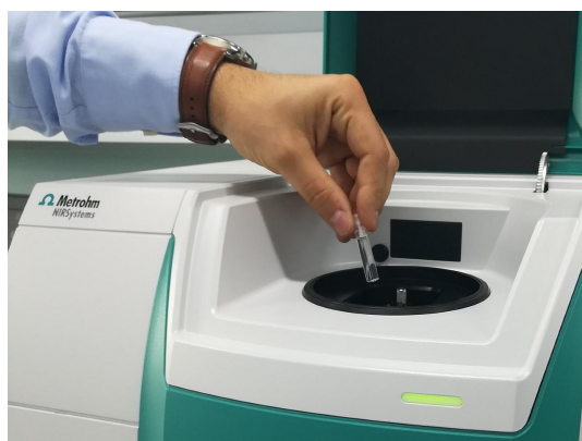
Figure 1. DS2500 Liquid Analyzer and a palm oil sample present in an 8 mm disposable vial.
