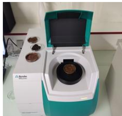
Figure 1. DS2500 Solid Analyzer with human stool samples.
