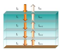
Figure 2. Normal reflection configuration.
