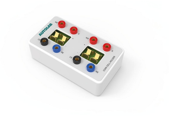
Figure 1. The Metrohm Autolab DuoCoin Cell Holder
