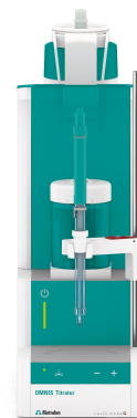
Figure 1. OMNIS Advanced Titrator equipped with a double Pt sheet electrode for the determination of ozone in water samples.
