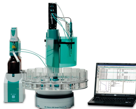
Figure 1. Titrando system consisting of an 815 Robotic USB Sample Processor XL in combination with a 907 Titrando.
