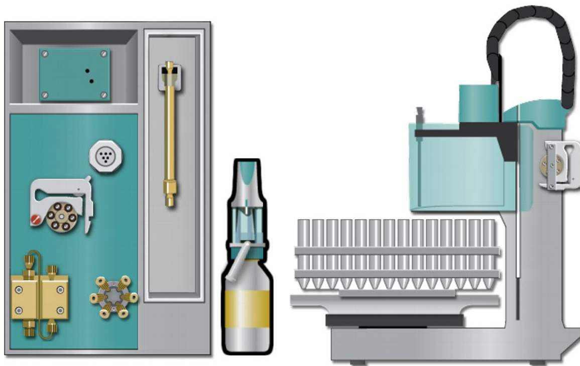
Figure 2. Compact instrumentation to quantify carbonate in sodium hydroxide: Compact IC Flex with a Dosino for MiPT and a 858 Professional Sample Processor.
