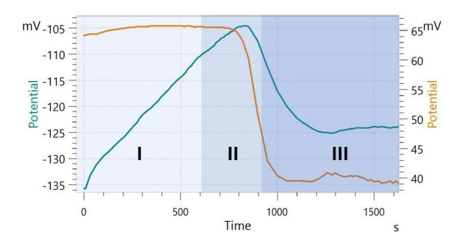
**Figure 2.** Example curve for calcium carbonate formation. In green is the potential of the free calcium ions measured with the combined Ca ion-selective electrode, and in orange, the potential measured with the Optrode. The experiment was carried out at pH 11. The colored phases describe the prenucleation phase (I), nucleation (II), and particle growth (III).
