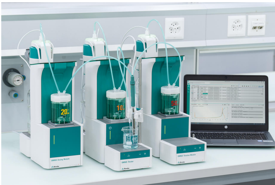
Figure 2. OMNIS Titrator equipped with a dPt Titrode electrode for the determination of caffeine content in aqueous samples.
