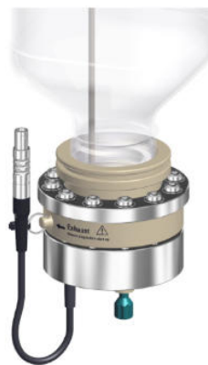
Figure 2. The 948 Continuous IC Module, CEP automatically produces KOH eluent from ultrapure water and a KOH concentrate. The electrochemical eluent production takes place at a membrane in the eluent producer cartridge.
