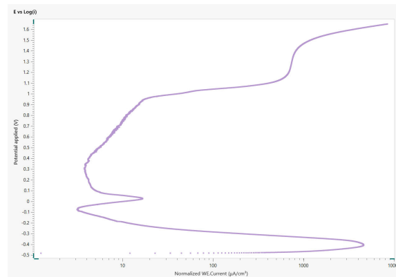
Figure 2. The corresponding plot of \log(j) vs E for the corroding sample of stainless steel in 0.5 mol/L sulfuric acid solution.
