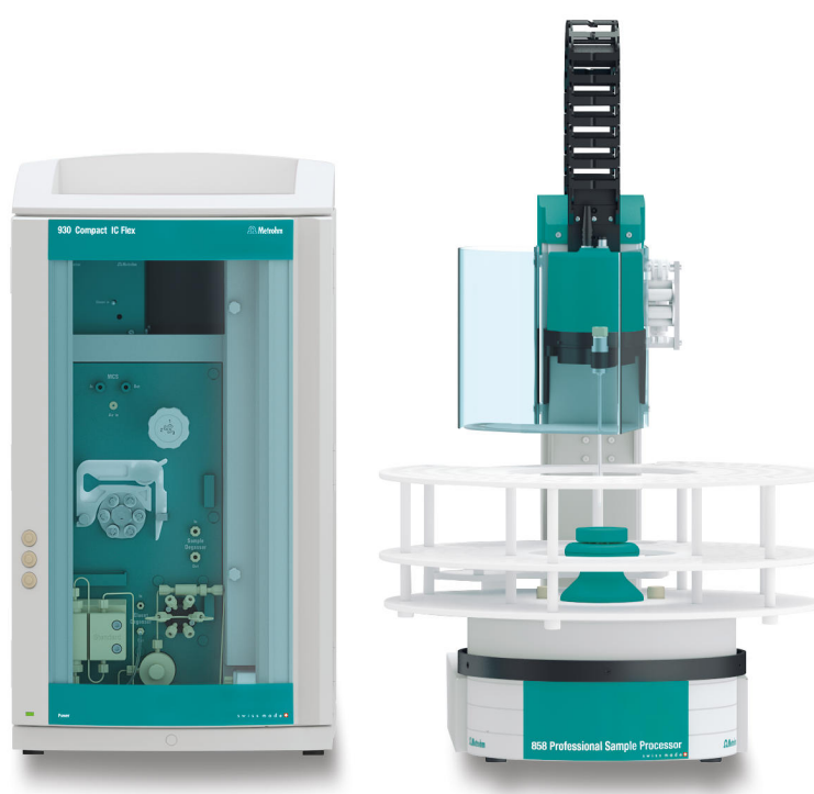
Figure 1. Instrumental setup including a 930 Compact IC Flex Oven/SeS/PP and an 858 Professional Sample Processor.
