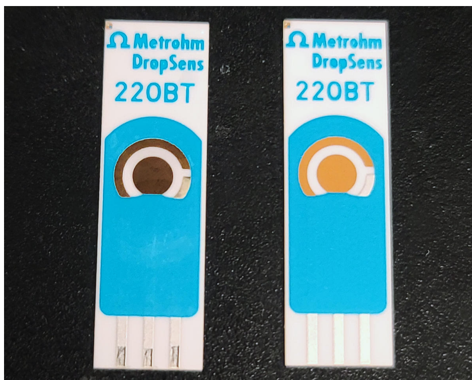
Figure 2. Surface of the WE before (left) and after (right) electrochemical roughening.
