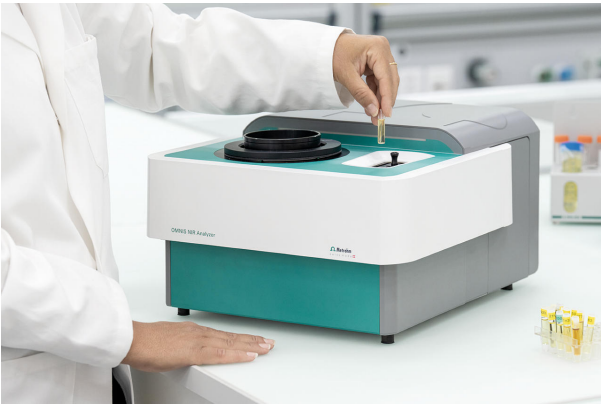
Figure 1. OMNIS NIR Analyzer and a sample filled in a disposable vial.
