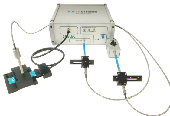
Figure 1. Fluorescence spectroelectrochemistry setup used for the study of Alamar Blue.
