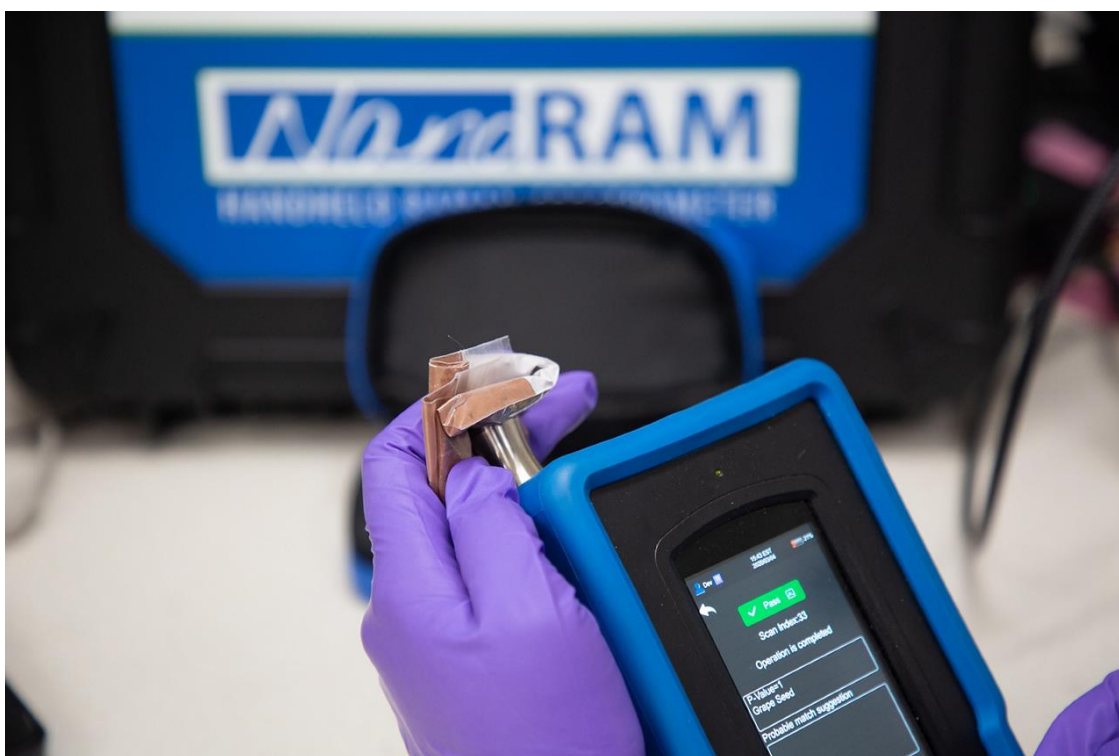
Figure 2. Analyzing grape seed extract with 1064 nm laser with point and shoot adapter.
