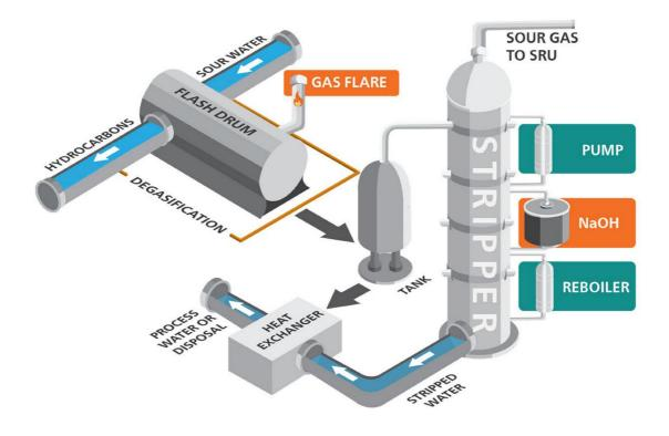
Figure 1. Sour water stripping process scheme (SRU: Sulfur Recovery Unit).
