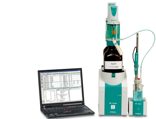
Figure 1. 905 Titrand with tiemo. Example setup for the determination of the iron content in iron ore.
