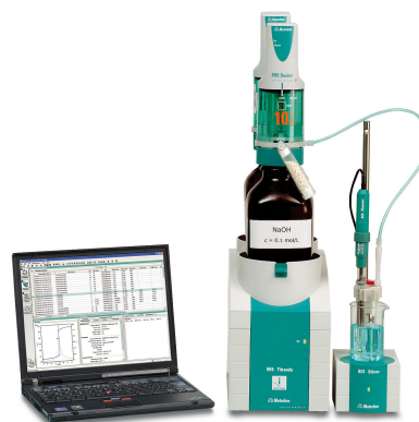
Figure 1. 905 Titrando with tiemo. Example setup for the determination of the titratable acidity in dairy products.
