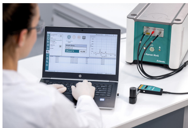
Figure 2. The i-Raman NxG combined with SpecSuite software is ideally suited for rapid detection and quantitative screening of dangerous adulterants in alcoholic beverages.
