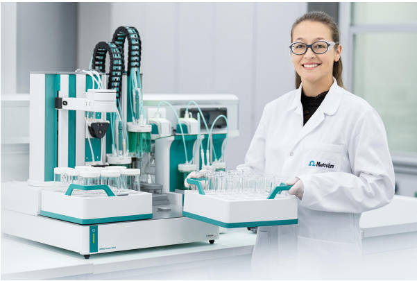
Figure 1. OMNIS Sample Robot and OMNIS Advanced Titrator equipped with a dUnitrode and Dis-Cover lids.
