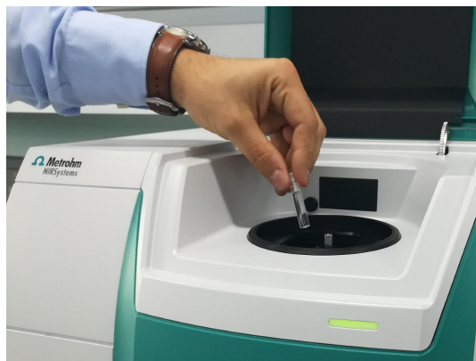
Figure 1. DS2500 Liquid Analyzer and a diesel exhaust fluid sample filled in a disposable vial.
