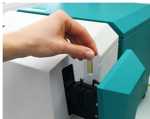
Figure 1. XDS RapidLiquid Analyzer and 8 mm disposable vial filled with a gasoline sample.
