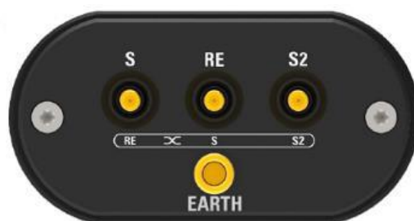
Figure 2. Shown here is the buffer box (part of the Pure Signal Bridge) with connections for the EARTH ground, as well as the Adaptive Cables of the sense (S), reference (RE), and second sense (S2).
