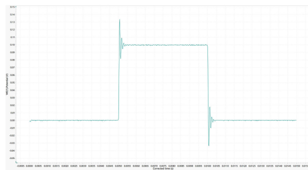
Figure 5. A positive feedback measurement of the circuit from Figure 1, dummy cell (c), with an acceptable iR compensation value of 95 \Omega .
