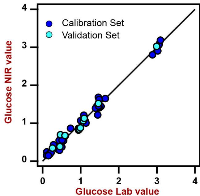
**Figure 4.** Correlation diagram and the respective figures of merit for the prediction of glucose content in an aqueous sugar mixture using a DS2500 Liquid Analyzer.
