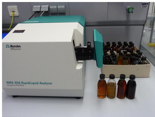
Figure 1. XDS RapidLiquid Analyzer and lubricant samples.
