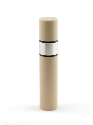
Figure 1. Rotating cylinder electrode showing the metallic insert, the Viton O-rings (black) and the PEEK holder.
