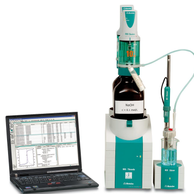
Figure 1. Titration system consisting of a 905 Titrand, a rod stirrer, and a Unitrode easyClean. The data are recorded and evaluated by tiamo.
