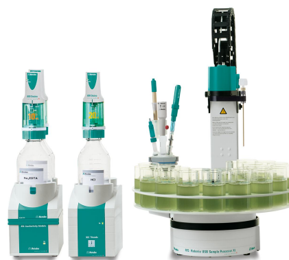
Figure 1. Example setup of a 815 Robotic USB Sample Processor XL with one external titration vessel, a 905 Titrandos and 856 Conductivity Module equipped with iAquatrode plus, combined Ca-ISE, iAg-Titrode, and 5-ring conductivity measuring cell for the analysis of tap water.
