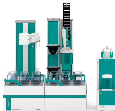
Figure 1. OMNIS System consisting of an OMNIS Sample Robot S and an OMNIS Advanced Titrator.
