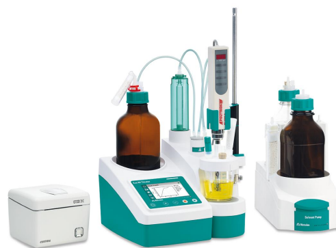
Figure 1. Eco KF Titrator equipped with a Polytron, a Solvent Pump, and a double Pt-wire electrode for volumetric Karl-Fischer titration.
