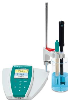
**Figure 1.** 914 pH/DO/Conductometer equipped with an O<sub>2</sub>-Lumitrode, conductivity measuring cell, and iUnitrode (missing in the picture) for the determination of DO, K (conductivity), and pH in liquid dairy products.
