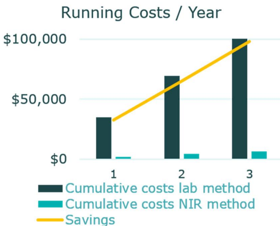
Figure 8. Comparison of the cumulative costs costs for the determination of key quality parameters in shampoo with titration/HPLC and NIR spectroscopy.
