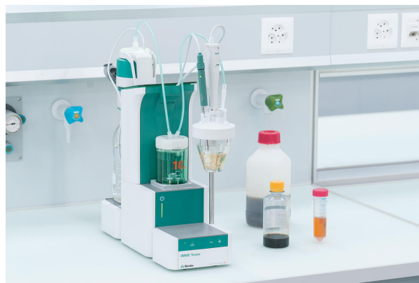
Figure 1. OMNIS Professional Titrator equipped with a dThermoprobe and a rod stirrer.
