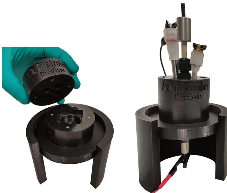
Figure 1. REFLECELL-C, the UV-Vis cell for conventional electrodes. Inner view (L) and completely assembled cell with WE, CE, RE, and optical fiber held with clamping piece for optimal positioning (R).
