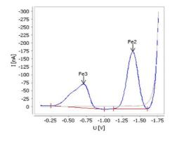
Figure 2. Determination of iron in iron sucrose injection
