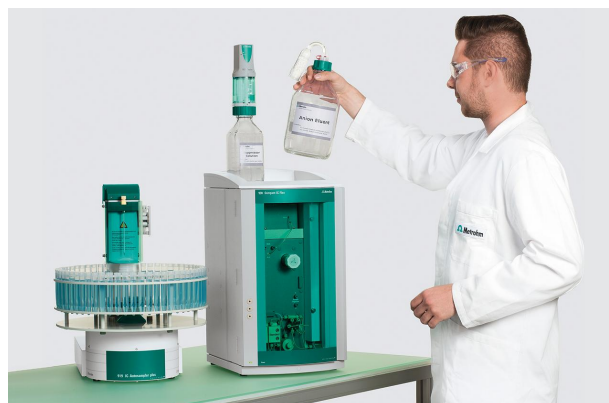
Figure 1. Compact, user-friendly Metrohm IC instrumentation to quantify various anions in explosives and explosion residues.
